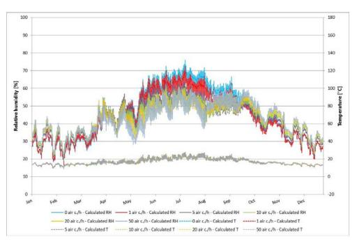
Chart 3: Position C. Calculated relative humidity and temperature with different applied air flow in the air gap. Different colors show different flow.
