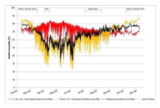
Chart 6: Example on comparison in position B. Measured relative humidity (black). Calculated relative humidity for 1 air changes per hour (read). Calculated relative humidity for 20 air changes per hour (yellow). Periods with gaps in boundary conditions are shown in the top.
