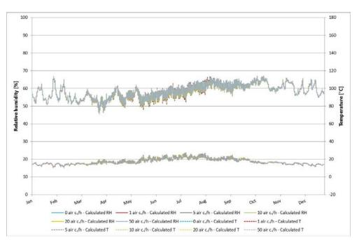
Chart 5: Position D. Calculated relative humidity and temperature with different applied air flow in the air gap. Different colors show different flow.
