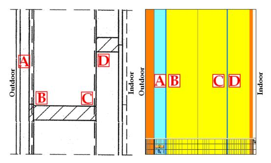
Figure 1: Drawing of estimated wall construction and WUFI 4.2 model. Air gap with different air flow for each calculation (A). Calculated positions (B, C and D).
